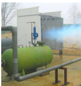
Safety valve test Bench
